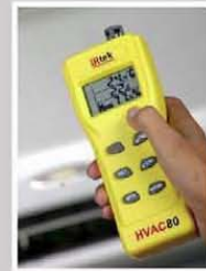
air temperature and humidity measurement
