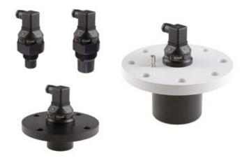
**Ultrasonic level meters ULM**<sup>®</sup> is self contained device that includes electroacoustics transducer and electronic module. The level meter ULM transmits series of ultrasonic pulses which propagates towards the liquid surface. Reflected acoustic wave is received back in the ULM transducer and processed in electronic module. The distance calculations are based on time of flight of the acoustic wave to the level and back.
