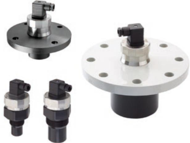
Ultrasonic level meters ULM® is self contained device, that includes electroacoustics transducer and electronic module. The level meter ULM transmits series of ultrasonic pulses, which propagates towards the liquid surface. Reflected acoustic wave is received back in the ULM transducer and processed in electronic module. The distance calculations are based on time of flight of the acoustic wave to the level and back.
