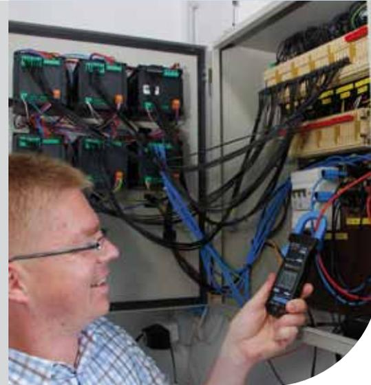
The MD 9225 is a versatile current clamp meter with perfect combination of size and built-in functions. It measures AC/DC current and voltage, capacitance, temperature, full range resistance and captures in-rush current. Display with large easy-to-read figures and one-handed operation make MD 9225 an extremely easy-to-use. This compact instrument combines a high level of functionality, small size and portability. All built-in features make MD 9225 a perfect tool for advanced applications.
