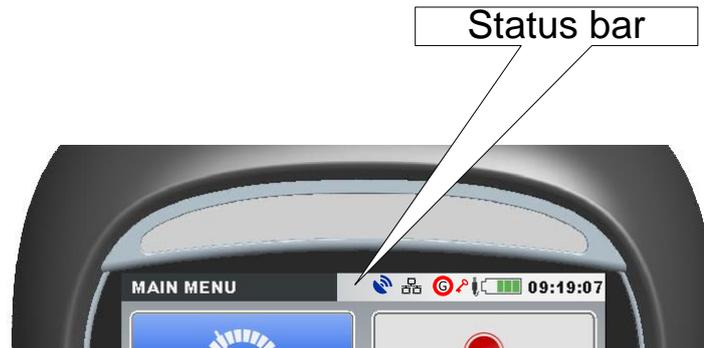
Figure 3.3: Instrument status bar
