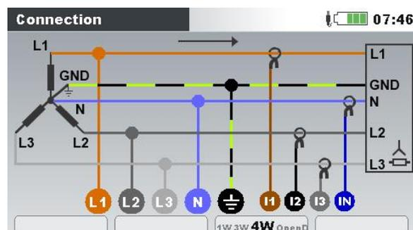
Figure 4.3: Choosing 3-phase 4-wire system on instrument
