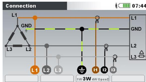
Figure 4.5: Choosing 3-phase 3-wire system on instrument
