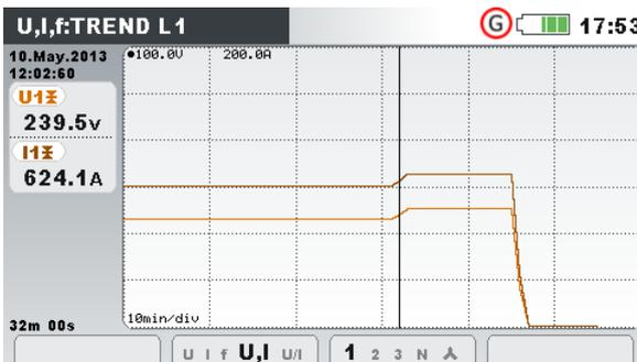
Figure 3.18: Voltage and current trend (single mode)
