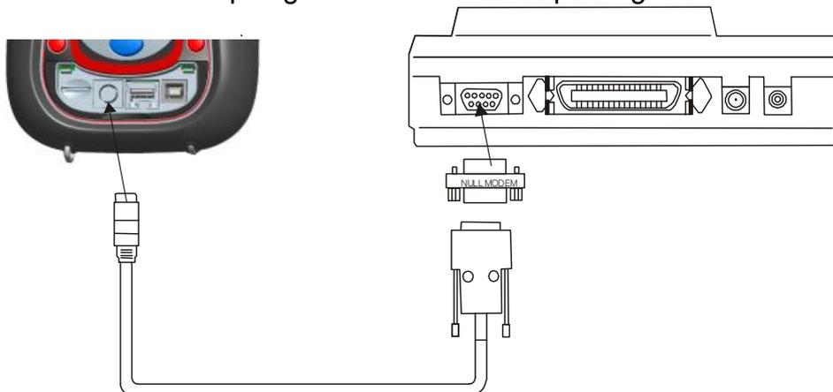
Figure 4.21: Connecting printer DPU 414 with instrument
