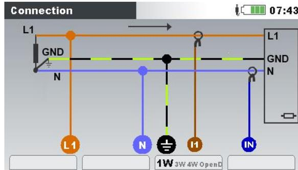
Figure 4.9: Choosing 1-phase 3-wire system on instrument
