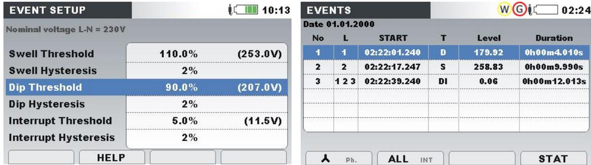
Figure 5.11: Voltage dip related screens on the instrument
