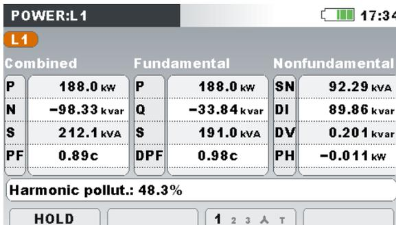
Figure 3.24: Detailed power measurements at phase L1
