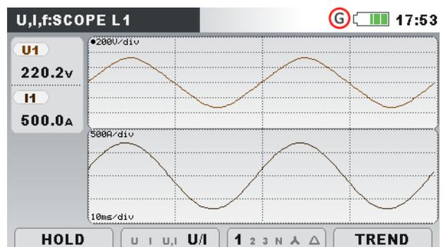
Figure 3.15: Voltage and current waveform (dual mode)
