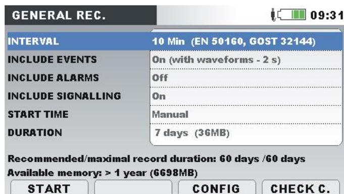
Figure 5.25: Predefined EN50160 recorder configuration
