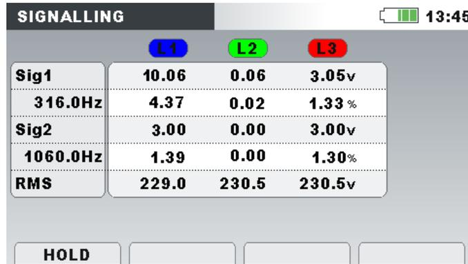
Figure 3.43: Signalling meter screen
