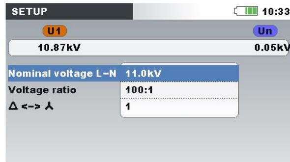
Figure 4.13: Voltage ratio for 11 kV / 110 kV transformer example
