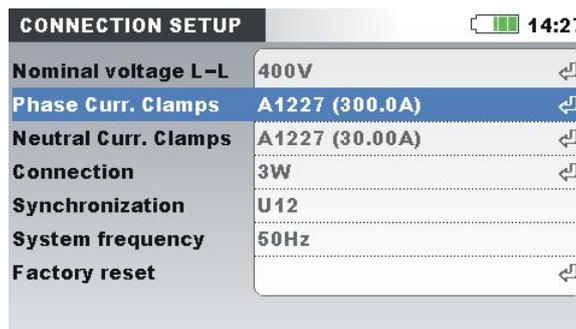
Figure 4.18: Automatically recognised clamps setup
