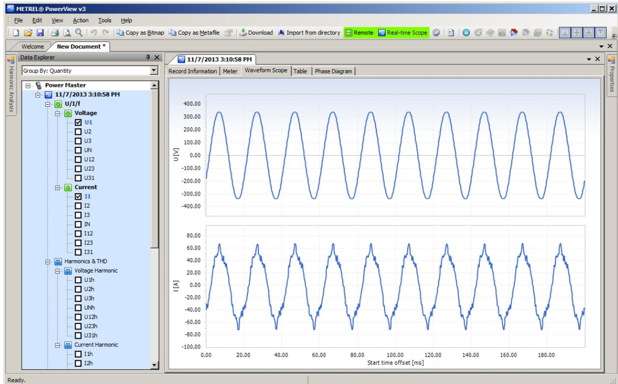
Figure 4.35: Real time scope window in remote connection, with several channels selected
