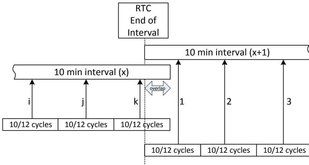
Figure 5.14: Synchronization and aggregation of 10/12 cycle intervals
