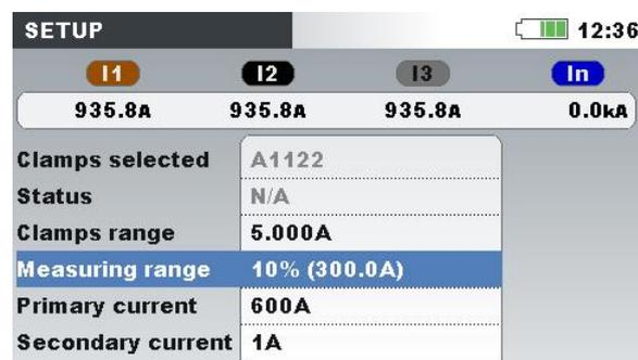
Figure 4.17: Selecting 10% of current clamps range
