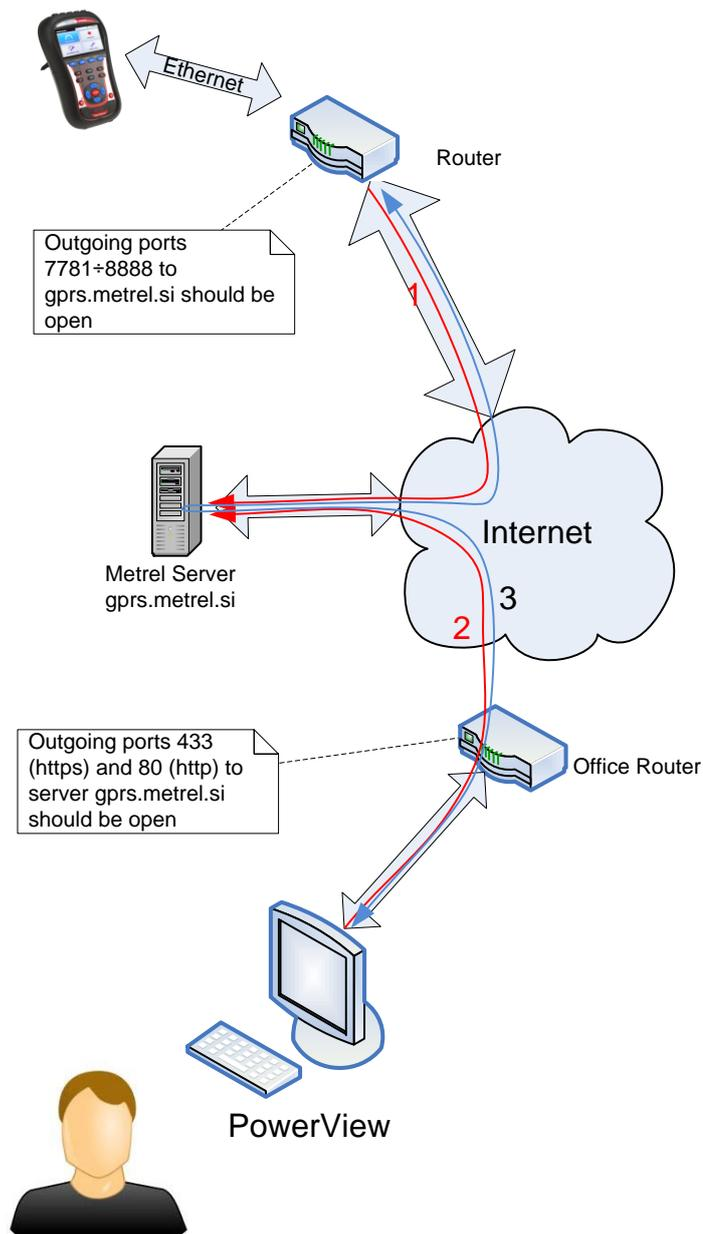
Figure 4.23: Schematic view on the remote measurements
