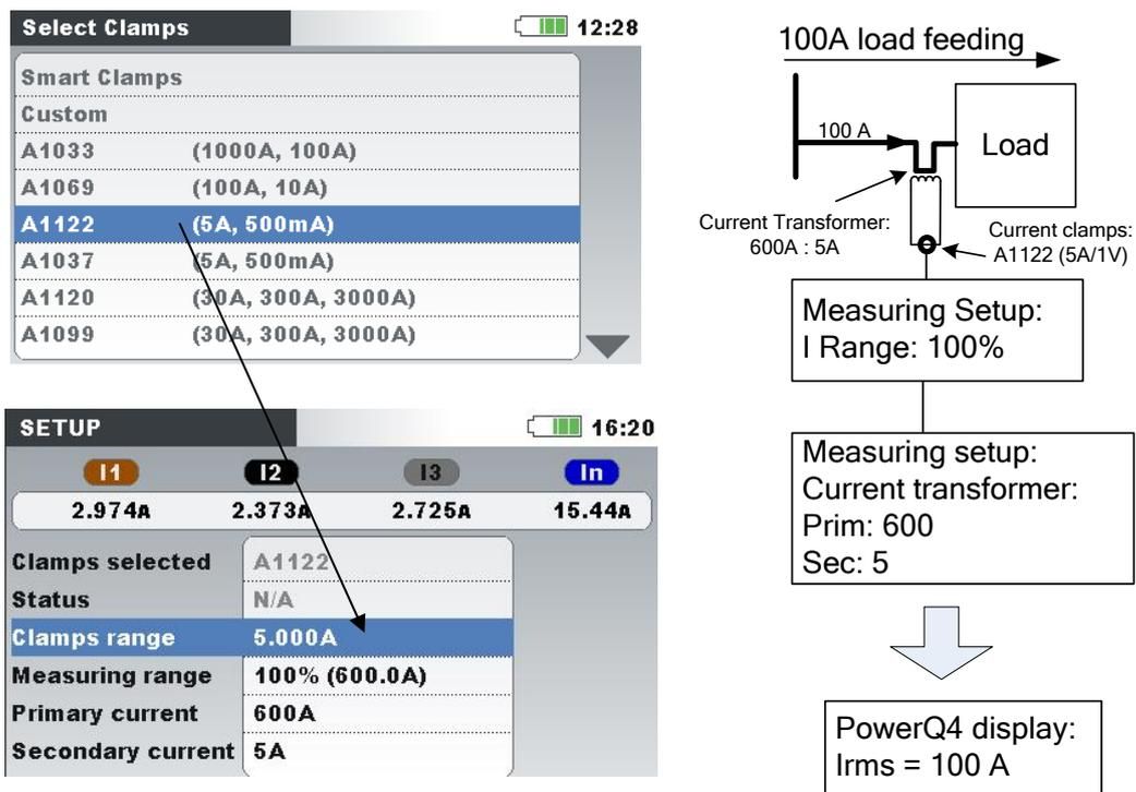
Figure 4.16: Current clamps selection for indirect current measurement
