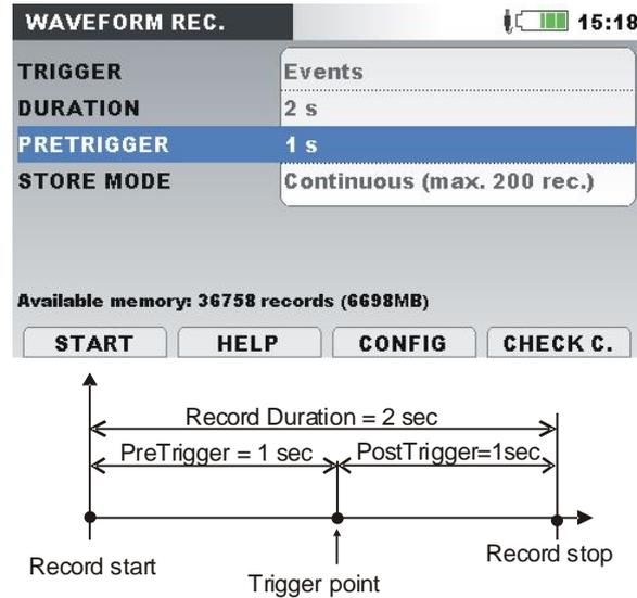
Figure 5.17: Triggering and pre-triggering description
