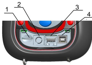
Figure 2.3: Side connector panel
