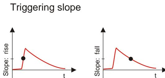
Figure 5.23: Triggering slope
