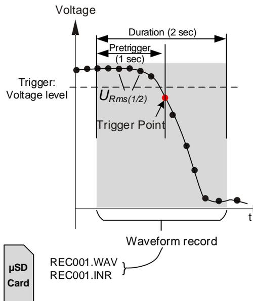
Figure 5.19: Voltage Level Triggering
