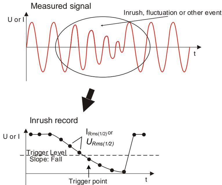
Figure 5.22: Level triggering
