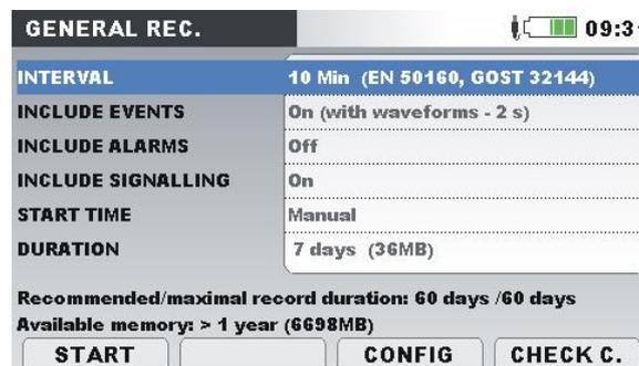
Figure 3.46: General recorder setup screen
