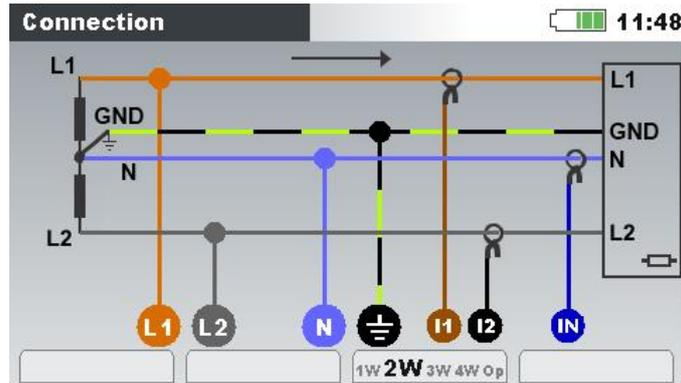
Figure 4.11: Choosing 2-phase 4-wire system on instrument
