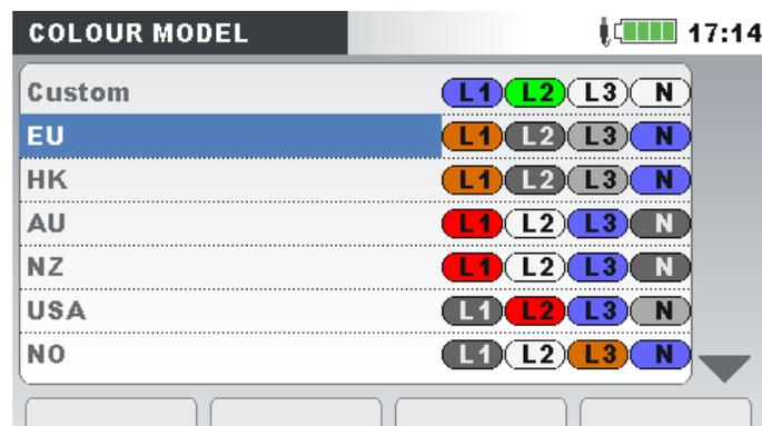
Figure 3.74: Colour representation of phase voltages
