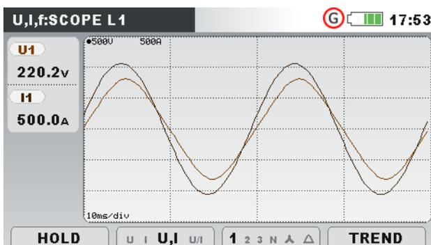
Figure 3.14: Voltage and current waveform (single mode)
