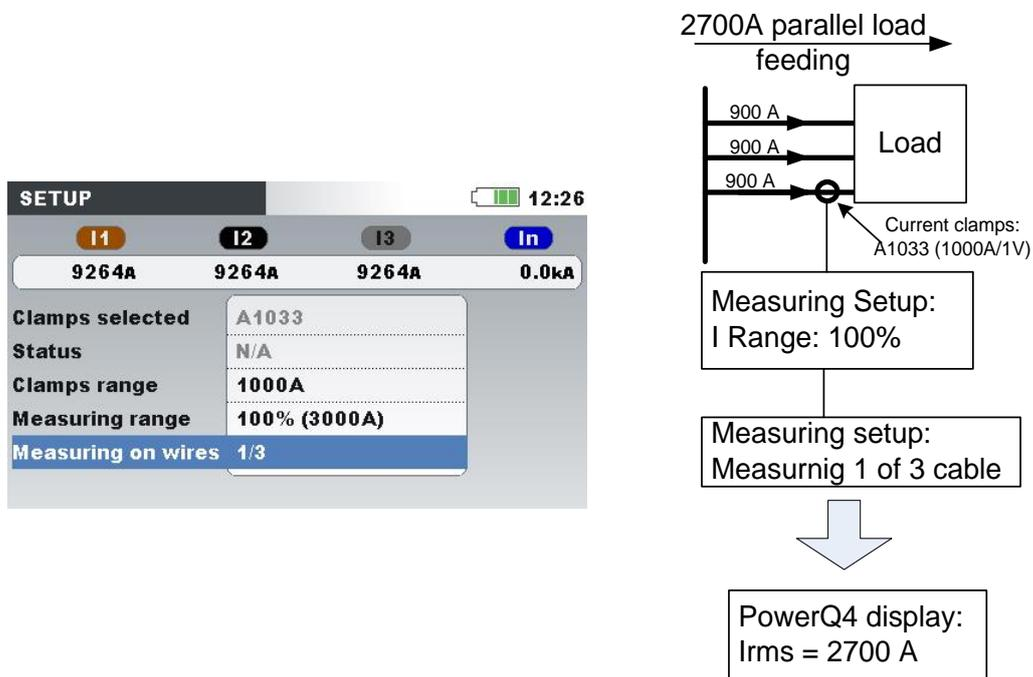
Figure 4.15: Parallel feeding of large load
