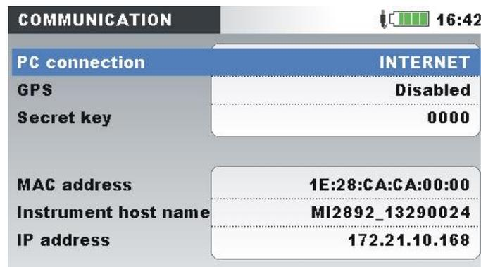
Figure 4.24: Internet connection setup screen
