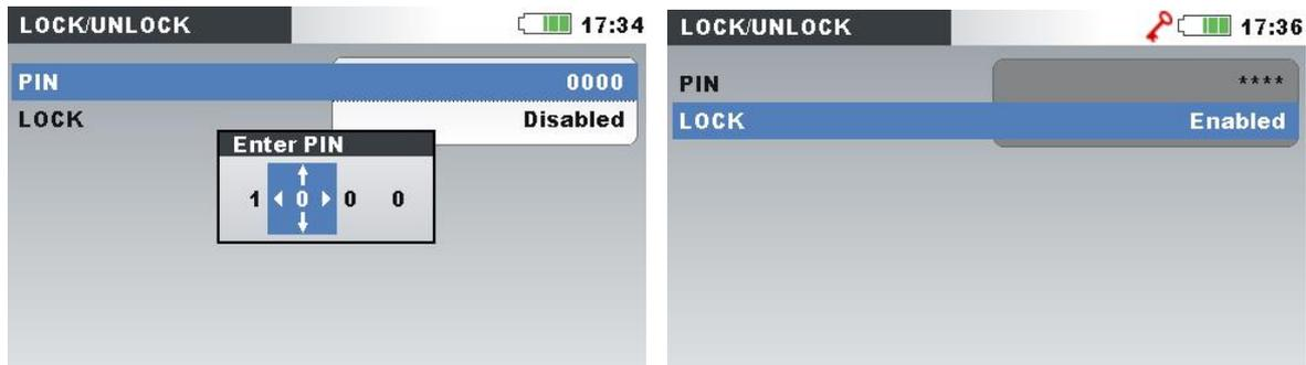
Figure 3.72: Lock/Unlock screen
