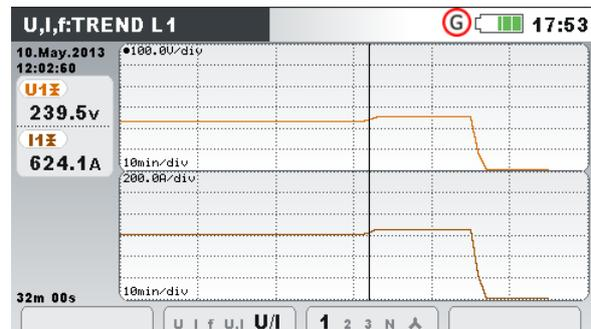
Figure 3.19: Voltage and current trend (dual mode)
