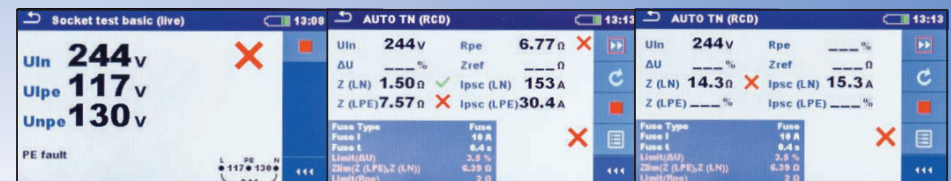
Earth Open Circuit FAIL Result
