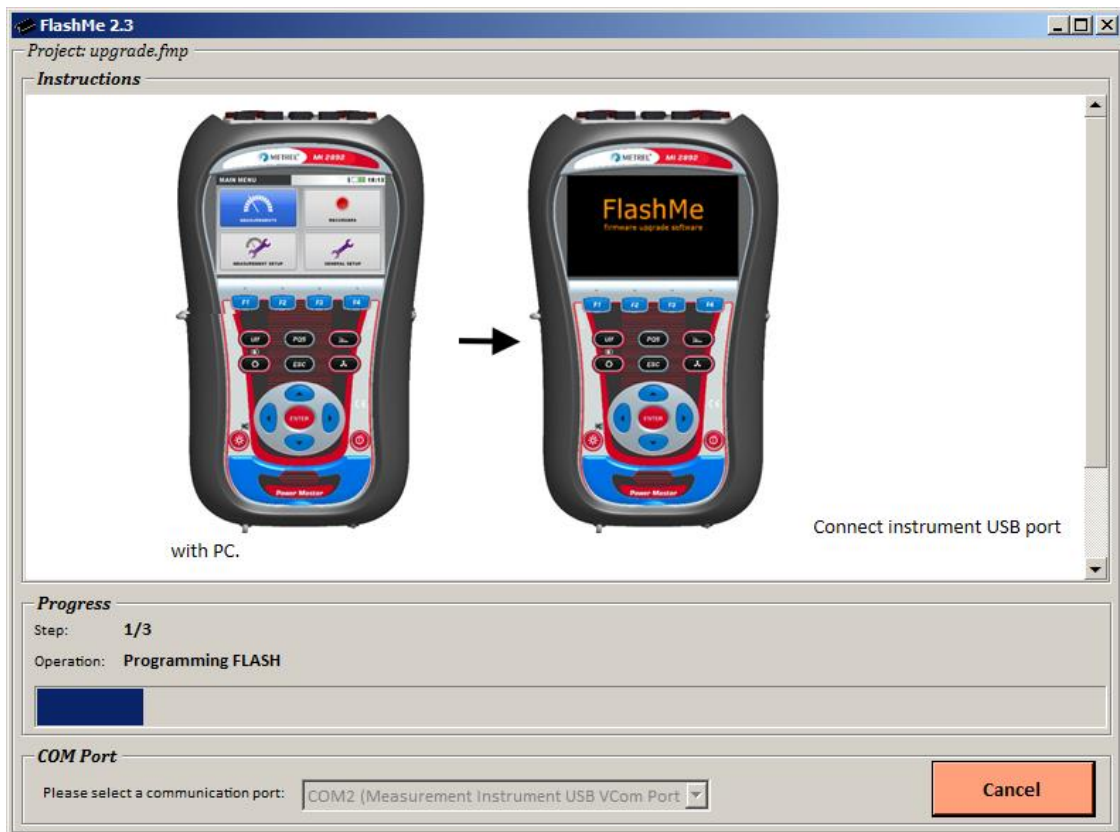
Figure 8.10: FlashMe programming screen
