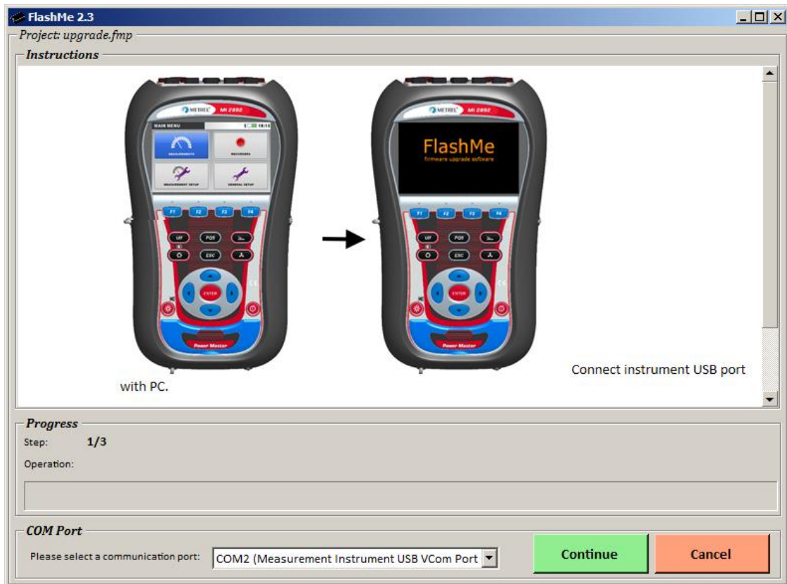
Figure 8.9: FlashMe configuration screen
