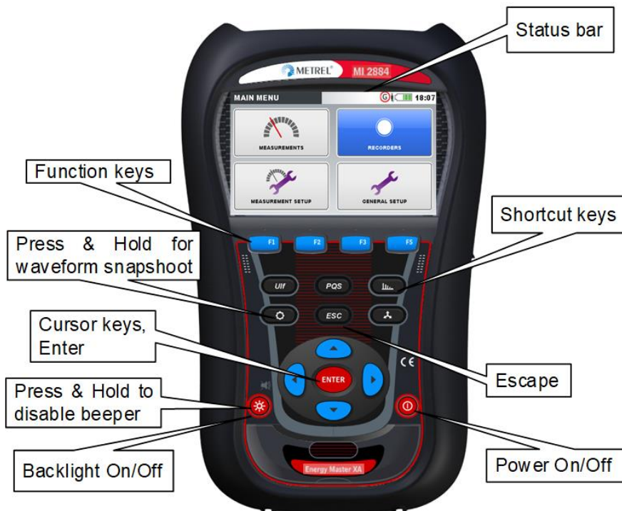
Figure 4.1: Display symbols and keys description
