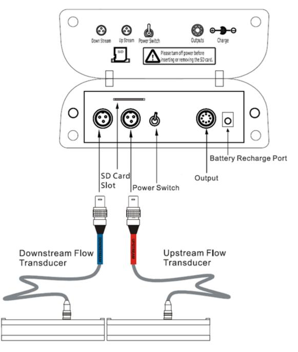
Turn on the power switch at the top of the meter, then you can proceed with using the flow meter. If it does not turn on it may need to be charged before use.
