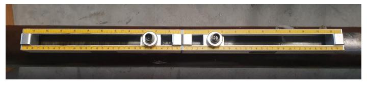
Rotate the transducer mount which is spring loaded to ensure the transducer is firm up against the pipe. This rotary knob moves the transducer in and out within the frame for a snug fit.
