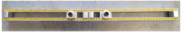
Apply couplant to both transducer sensing surfaces, like in the below example:
