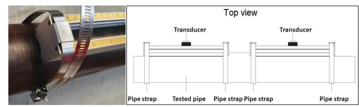
Hint: in some situations, it might be easier for you to use only one frame, you could remove on transducer and place it into the other frame with it if you will always be using V method on small pipes
