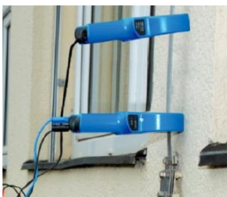
Many optional accessories like current clamps for leakage and conductive loops
