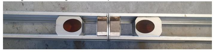
After setting all the previous correct parameters, space the transducers as per the distance on menu 25
