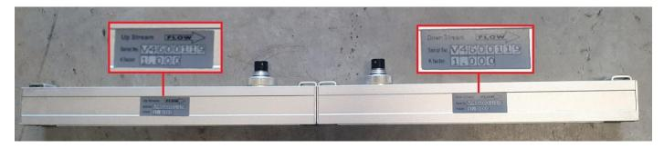
On each transducer you will also see and upstream or downstream marking to ensure it is in the relevant frame.
