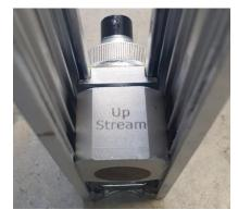
Also note that when looking at the bottom of the frames in when in the correct orientation, the brown oval which is the sensing surface should be facing each other like below picture when used in V method.
