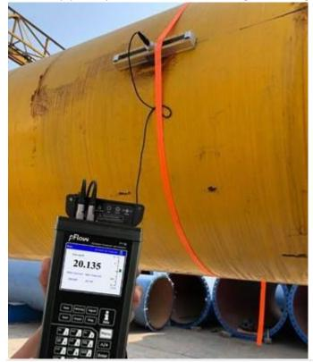
Hint: in some situations, it might be easier for you to use only one frame, you could remove on transducer and place it into the other frame with it if you will always be using V method on small pipes
