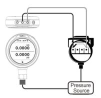
Figure 13 Calibrate pressure transmitter
