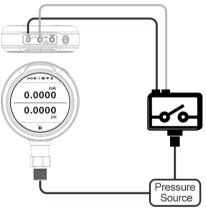
Figure14 Calibrate Pressure Switch
