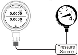
Figure 12 Calibrate Dial Pressure Gauge
