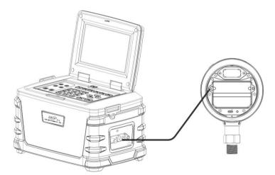
Figure 11 Barometric calibration
