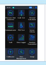
The onboard applications provide a useful selection of features including HART communicator, high static differential pressure mode, pressure leak test, safety valve test, analog transmitter calibration, unit converter, thermal calculator, and snapshots to name a few.
