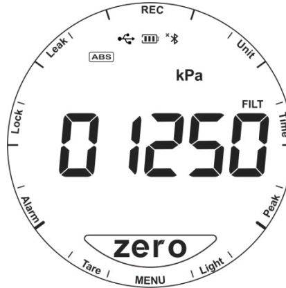
Figure 3 Main Operation Interface
