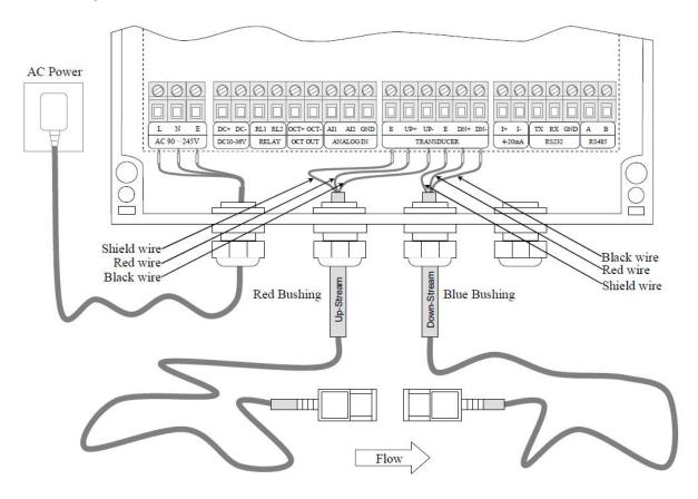
Please wire in all cables and ensure that all cables are run through the supplied cable glands and tightened up to prevent dust and water ingress.
