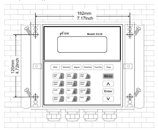
There are flip open covers on the left and right side which when opened expose the screws to open the enclosure and the holes/mounting points for wall mounting.
