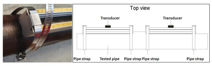
Hint: in some situations, it might be easier for you to use only one frame, you could remove on transducer and place it into the other frame with it if you will always be using V method on small pipes
