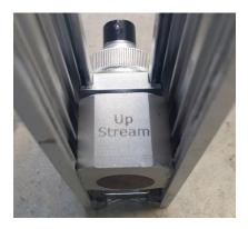
Also note that when looking at the bottom of the frames in when in the correct orientation, the brown oval which is the sensing surface should be facing each other like below picture when used in V method.
