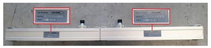
On each transducer you will also see and upstream or downstream marking to ensure it is in the relevant frame.
