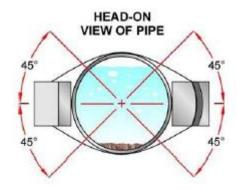
Now that you know how far to space the transducers apart from the previous step, and you have selected a suitable location for the installation with enough distance upstream and downstream away from bends, pumps, valves etc... you can prepare the pipe for mounting the transducers.
