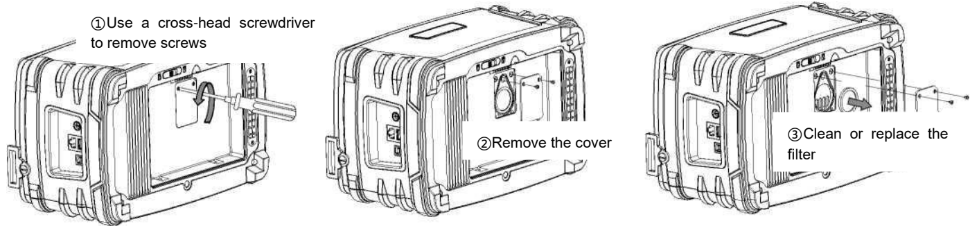
Figure 8- 1 Disassembly of the suction filter
