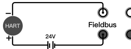
Figure 17 HART external power / internal resistance
