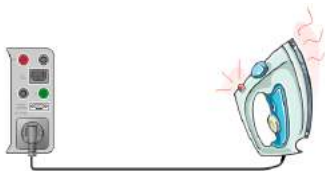
Differential leakage current test for Class I device
