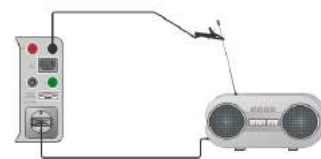
Substitute leakage test for Class II device
