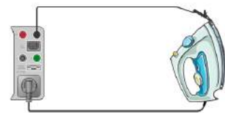
Substitute leakage test for Class I device
