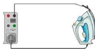
Earth bond test
