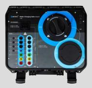
The A 1832 Mode 3 Charging cable adapter is used for electrical safety testing of Mode 3 EV charging cables with Type 2 connectors together with supported METREL or third-party testers. If used together with Metrel AutoSequences®, integrated in the newer multifunctional testers, the EV charging cable can be comprehensively tested (including functionally) with a push of a button. It is possible to create a professional report using MESM software.
