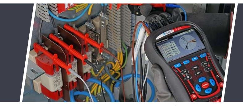
The Metrel power quality (PQ) analysis range allows automatic voltage/current and thus power quality analysis. They can be used as a maintenance and troubleshooting tool to discover transients, resonant states, high neutral conductor currents and asymmetric harmonics. All models can be used as power loggers or PQ meters.
