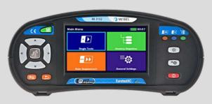
The MI 3152 multifunction installation tester offers complete installation safety testing (according to AU/NZ 3017) that comes with pre-defined auto sequence testing of TN, TT and IT earthing systems. A wide range of functions are included: from on-line voltage monitoring, phase sequence testing, insulation testing, earth measurement, to RCD tests, line and loop impedance tests and more.
