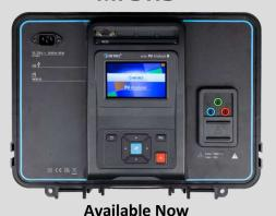
MI 3115 can test insulation resistance at 1500 V for solar strings, continuity of conductors, polarity, Isc & Voc and capture of irradiance and cell temperature of the PV modules wirelessly via the remote unit.
