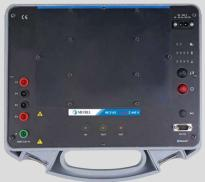
The **MI 3143** is intended for measuring the effectiveness of automatic trip out protection in case of faults in transformers and other HV equipment.
