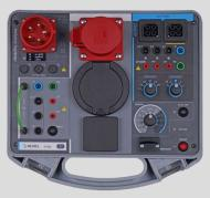
The A 1632 is a different kind of instrument. It is designed to thoroughly test the charging station on both the installation and the output sides. It can test Mode 2 and Mode 3 cables and monitor communication between station and car. Rather than for periodic testing, it is meant for installation tests and equipment producers. Professional reports for both station and cable status can be created in Metrel electrical safety management software (MESM).
