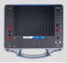
The MI 3144 is a high precision 4 wire, 300 A Loop and Line impedance testing. High range 800 V/16 to 420 Hz impedance measurements and DC sourcing and line resistance measurements from 3 to 260 V. Test earth leakage relays trip out time and current, partial voltage drops, current path resistances and ground fault analysis with contact, touch and step voltage. Can be used as a stand alone device with Android app A 1522 aMESM or in conjunction with various Metrel Multifunction testers.
