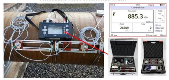
The UW-30P portable, clamp-on ultrasonic flowmeter provides instantaneous flow rate measurements with up to 2 pairs of transducers placed on the outside of pipes.
