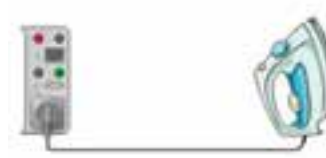
Insulation resistance test for Class I device
