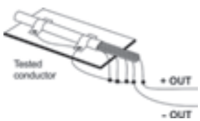
Measurement of insulation resistance between one lead of communication cable against other leads and sheath
