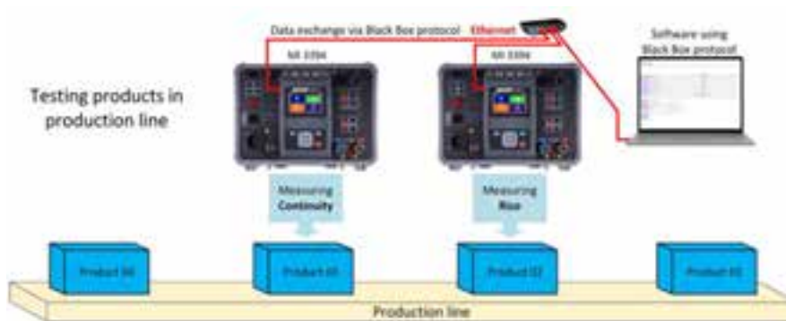
Product line testing using Black Box protocol for data exchange
