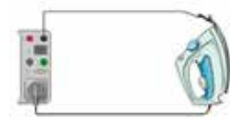
Substitute leakage test for Class I device
