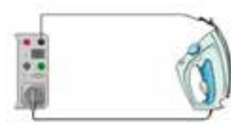
Earth bond test
