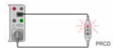
Active polarity test
