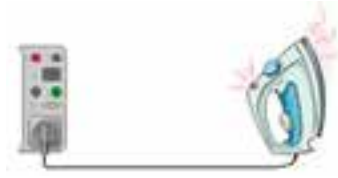
PE conductor leakage current test for Class I device
