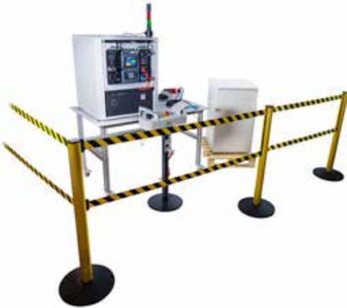
S 2111 safety system with Two hand control
