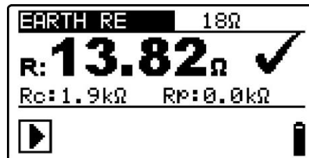
Figure 5.35: Example of earth resistance measurement result
